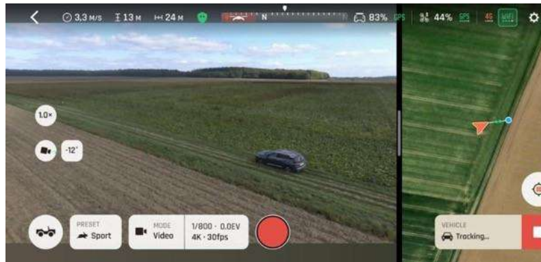
Tracking in progress, no command from the pilot: ANAFI Ai is travelling as the same speed as the vehicle
