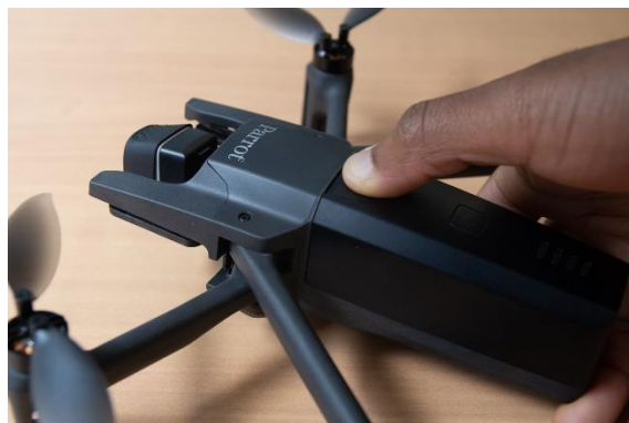
ANAFI Thermal: battery removal
