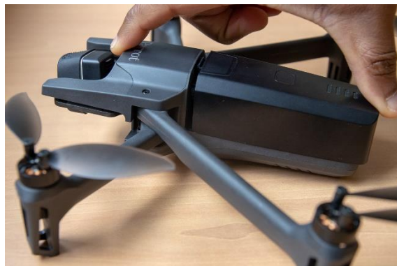
ANAFI Thermal: battery installation
